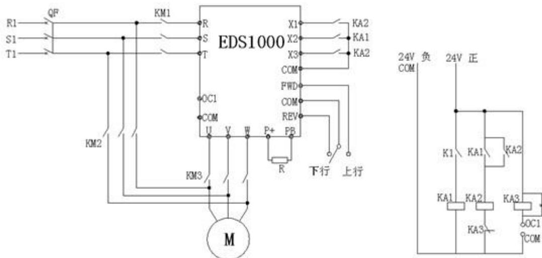
**Fig 2. Electric Wiring Diagram**
